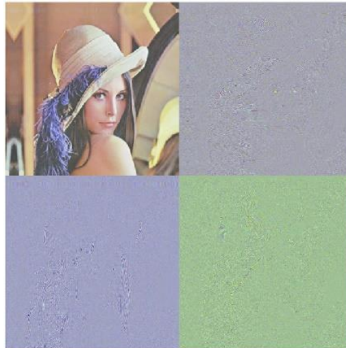
Figure 1. First Order Decomposition Wavelet Transform
